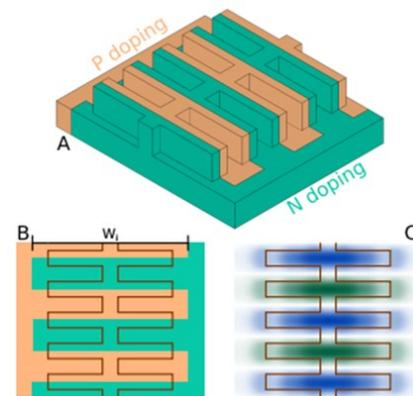
Slow Light Modulator and Interleaved PN junction: 3D view (A) and top view (B). Field profile of the optical mode (C).
