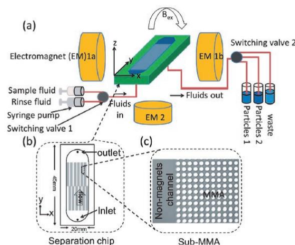
The flow enhanced non-linear magnetophoresis system (FNLM)
