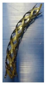
Figure 2 Morphing lattice with a curved deployment path
