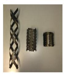
Figure 1: Three lattices with different stability point locations
